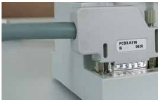
PCD3.K106/116 cable, hardware version B, with 90° angled connector
